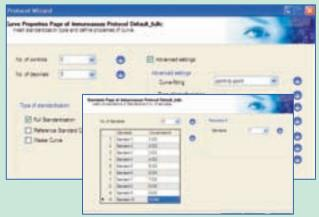
For more sophisticated curve fitting the full Immunoassay evaluation option offers additional algorithms such as cubic spline, linear regression and 4PL. In addition the alternative axis transformations log/log and logit/log can be applied.
